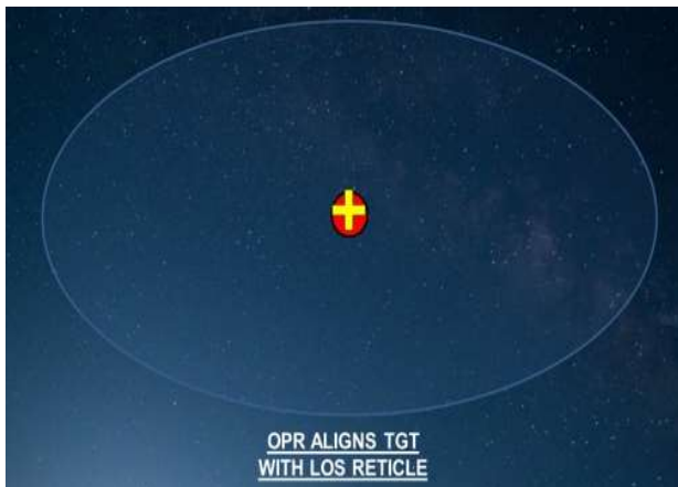
Fig 3 : Operator aligns target blip with the LOS reticle so that he is looking directly at the tgt. All this while, computer is calculating instantaneous position of target relative to firer.
