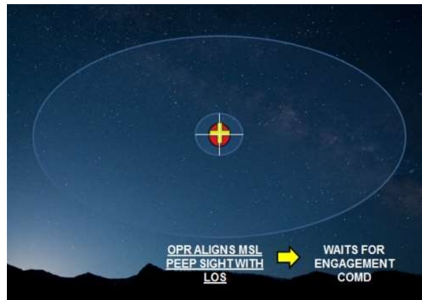
Fig 4 : Operator now aligns the Missile Peep Sight/ Gun Sight Crosshairs with LOS & keeps tracking the blip while waiting for engagement cmd.
